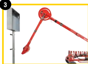
3 Align with conduit, properly adjust booms
